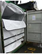
The anti-bulging mechanism provided inside the liner will prevent it from bulging. It has been tested by filling 25tons of material in a 20ft container and tilting it. Anti-bulging liners are available for 20ft, 30ft and 40ft containers.
